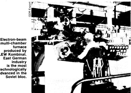
multi-chamber produced by LEW Kombinat. East German industry is the most technologically advanced in the Soviet bloc.
