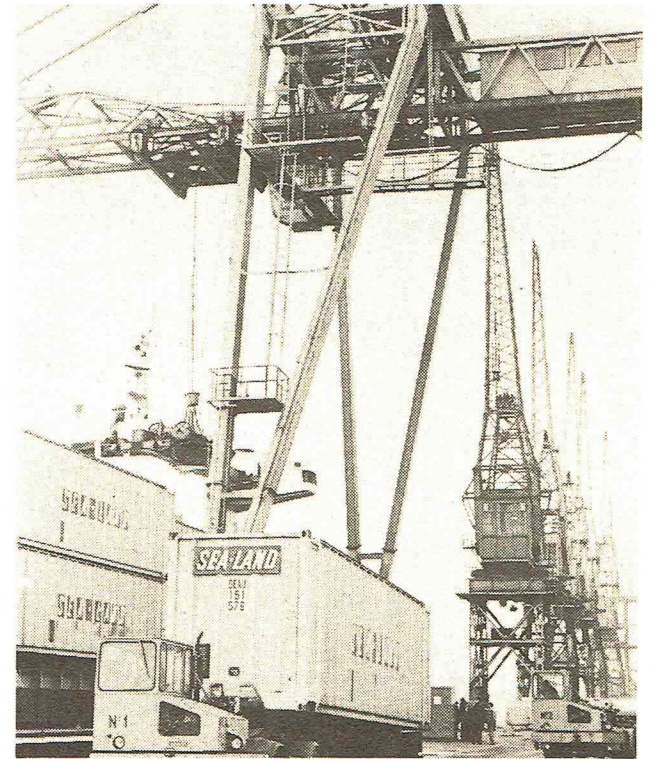
4,000 tons in containers takes eight hours to unload—before it would have been a week's work. But sometimes the traditional method still has to be used.
