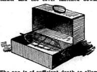
The pan is of sufficient depth to allow of the turning of the cage, roast and all, within the pan, the iron center rod reaching through the outside and one end of which is turned into a handle.
