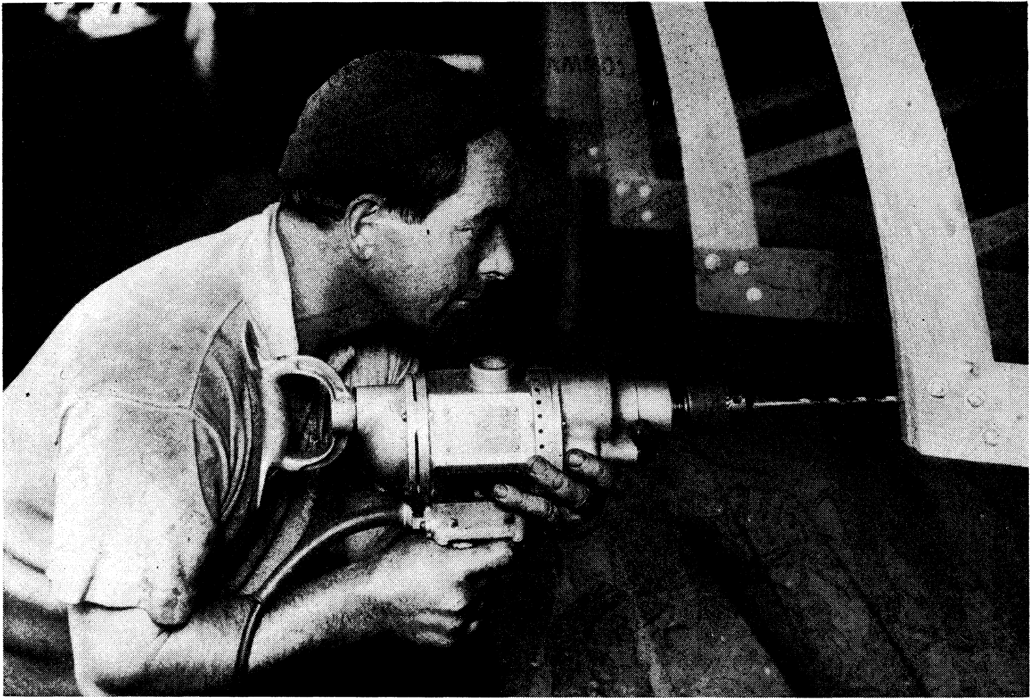
Finishing the frame for a Navy speed boat
