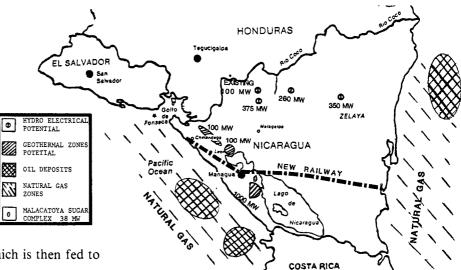
Nicaragua's first step on the road to energy self-sufficiency became a reality in early August, 1983, when a huge single turbine of the new 35MW (mega-watt) Momotombo geothermal energy plant turned for the first time under the force of naturally generated steam. The steam is produced from underground water which comes into contact with high-temperature rock. Wells
