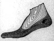
The new invention consists of the insertion of a mattress of canvas in which is embedded side by side a layer of narrow, flat, steel, springs. The canvas holds them in the pocket, in which they slide freely, but the ends are capped with metal to prevent their perforating the rubber and leav-
