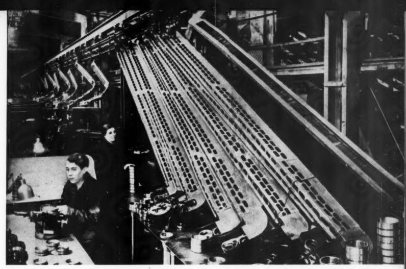
SOME 1,500 AUTOMATED AND CONVEYORIZED LINES FOR VARIOUS PROCESSES WERE INTRODUCED IN SOVIET INDUSTRY IN 1956. THIS ONE IS IN A BALL-BEARING PLANT.
