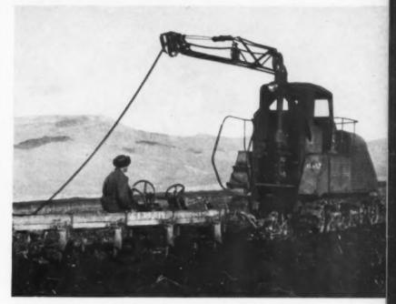
Electric-powered tractor used in plowing is one experimental farm technique. Cheap current from government-owned stations make this system economical.
