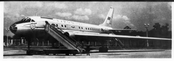
The TU-104A jet airliner carries seventy passengers and has a cruising speed of 550 miles per hour. It is one of several new types manufactured by Soviet industry for civil airlines. Among the new turbo-prop planes is an airliner that carries 200 passengers and cruises at 600 miles per hour.
