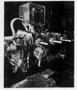
Many displays are dominated by automation and electronics. The tool shown here is designed to form six-crank shafts of different configuration.
