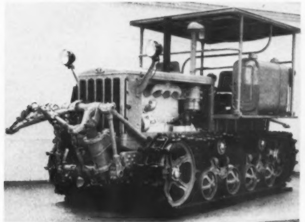
DIESEL TRACTOR EQUIPPED WITH POWERFUL HYDRAULIC LIFTING ARMS
