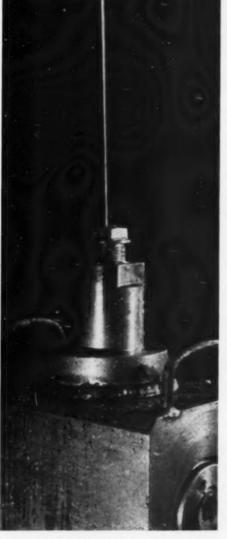
Electrohydraulic effect in this pump produces a jet of water which is able to cut through wood.
