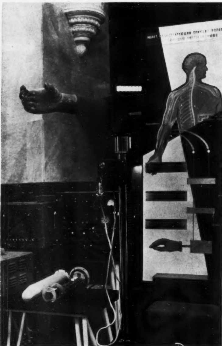
A glimpse into the exciting future for industrial automation will be provided by this mechanical hand, whose movements are directed by biocurrents of the human body through a transducer-amplifier assembly.
