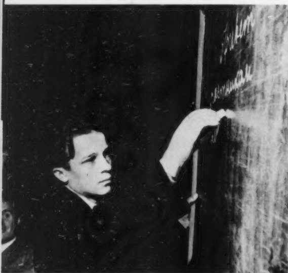
The young man is writing with a metal hand that is actuated by biocurrent signals from his brain.
