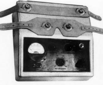
A portable "electric sleep" unit for use by surgeons, psychiatrists and therapists. Electrodes are placed on the patient's eyes and back of the head. They inhibit the nerve cells, produce a drowsy state and then sleep. In most cases the patient keeps on sleeping after the current is turned off.
