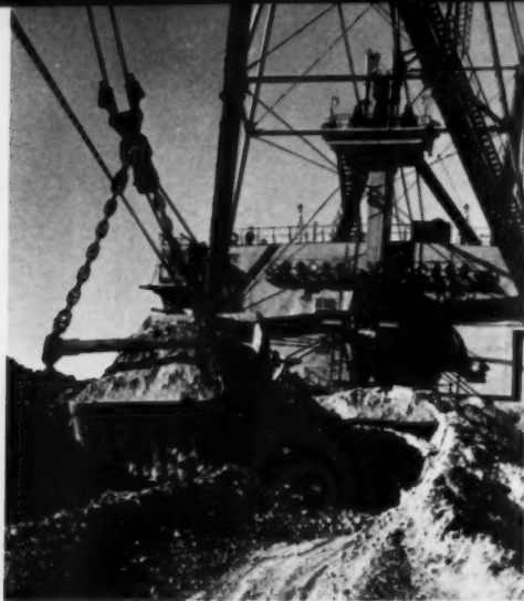
The bucket of this walking dragline used for open-cut mining can hold a ten-ton truck comfortably.
