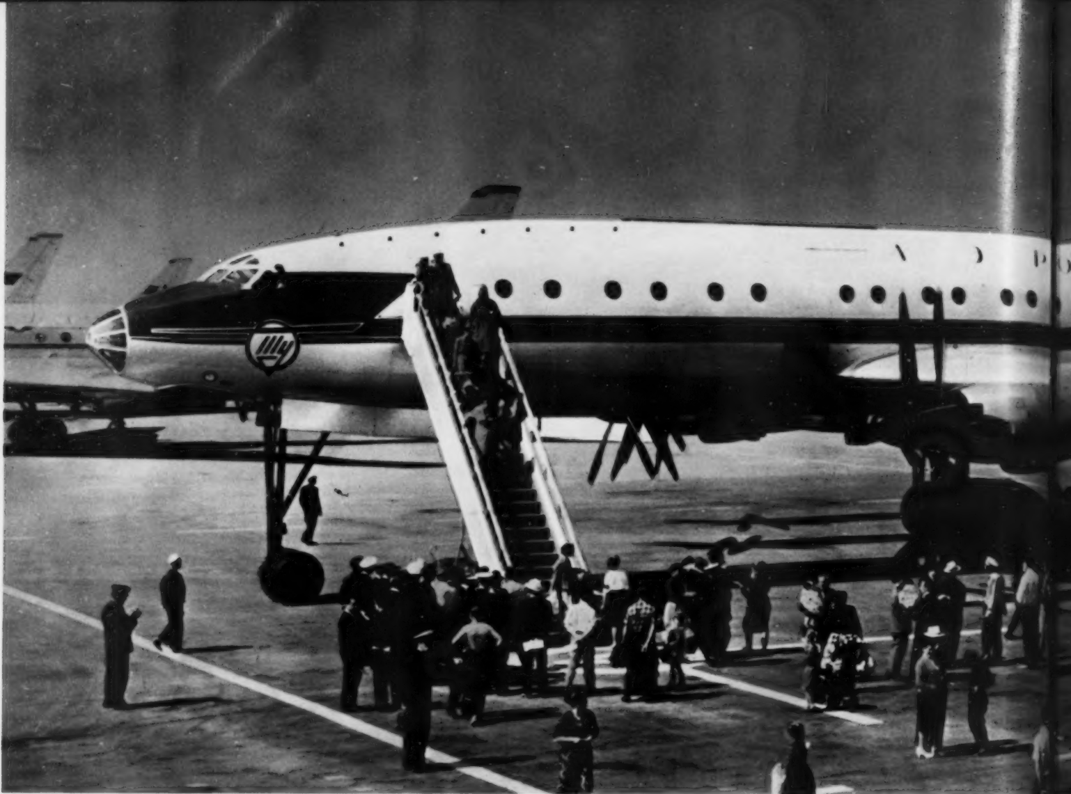
The turboprop giant TU-114 carries 170 passengers a distance of 4,350 miles nonstop in nine hours. Fares on the TU-114 and other big Soviet liners are no higher than for rail travel.
