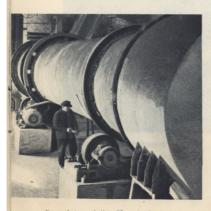
Granulator of the Shansi plant. It is used for making granular phosphate fertilizer
