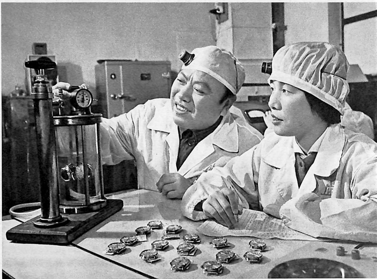
Testing the waterproofing. Wang Chia-teh (left), one of the workers who made the first batch of watches is now a technician.
