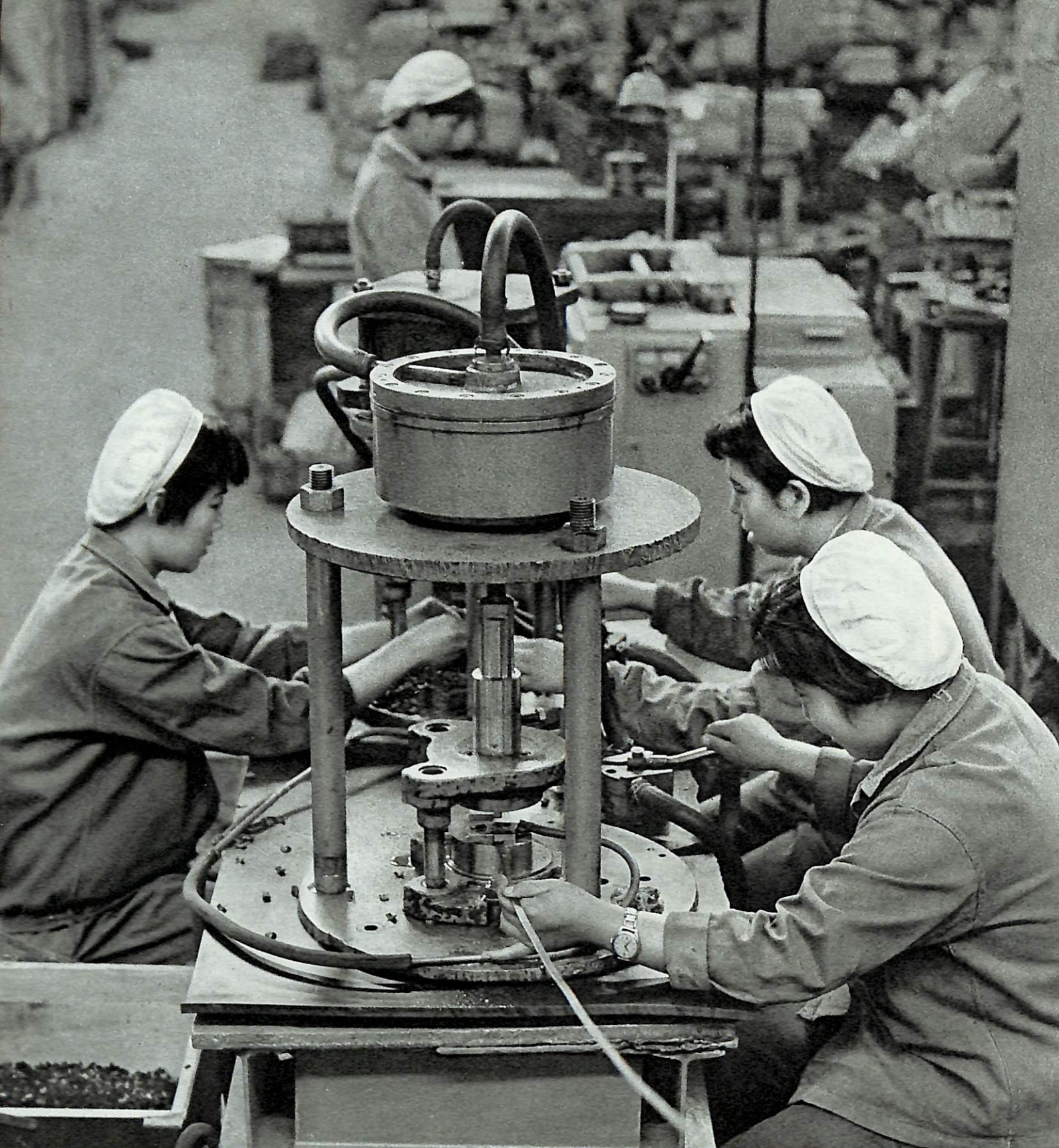
Sets of equipment made by the workers for machining the air-gate lock plate.
