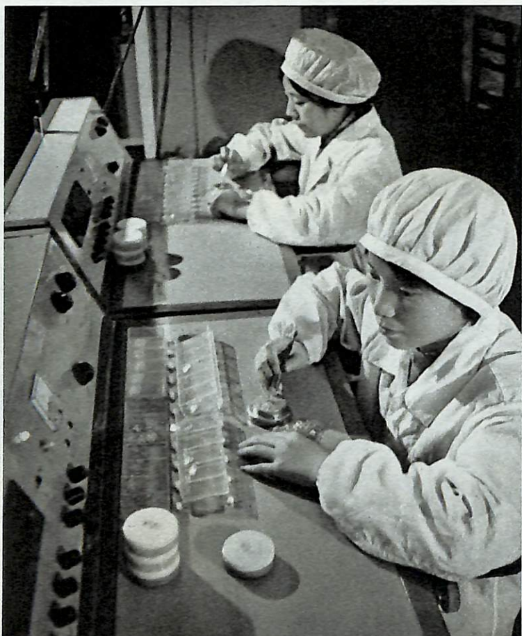
An instrument made by the workers for examining the balances and hair springs.
