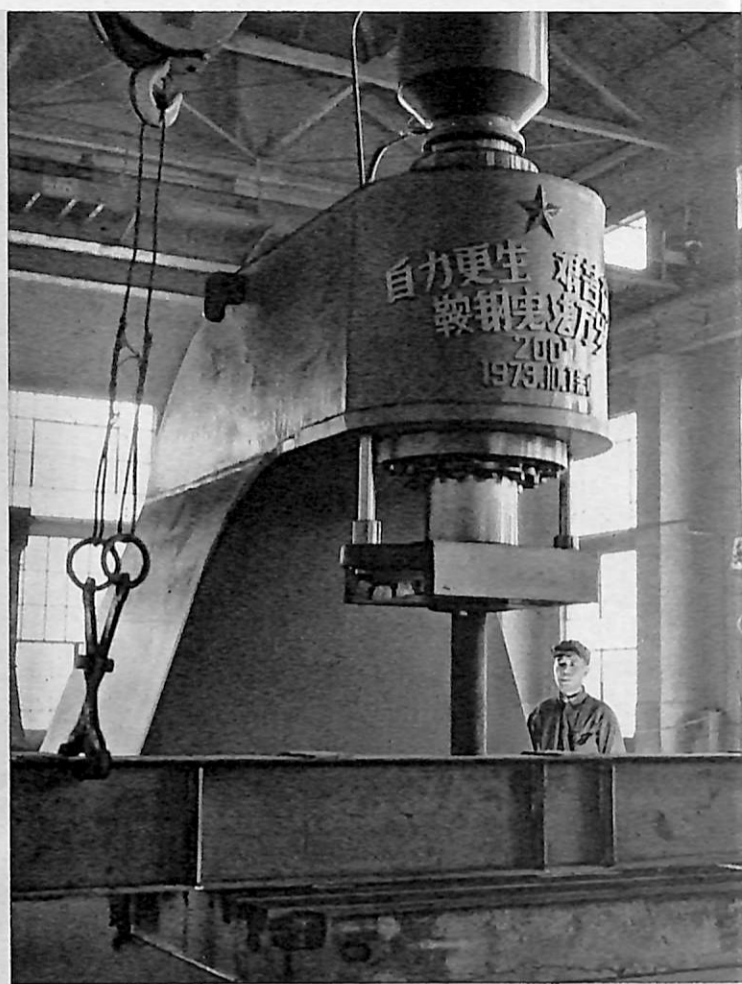
Mu Chin-kuei, a riveter, has made 60 technical innovations, aided by other workers and technicians. Here he is adjusting a component part of the oil pump with a 200-ton oil-pressure press designed by himself.
