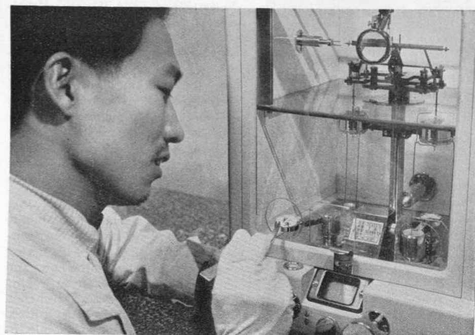
The ultra-sensitive microbalance.
