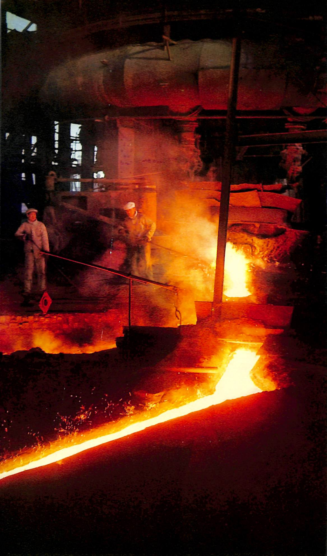
Molten iron flows from the No. 9 blast furnace.
