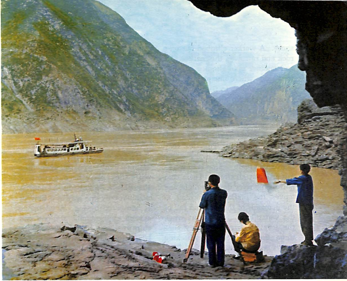
An advanced party of surveyors maps the depth of the river so that hazards can be removed.
