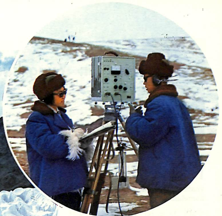
Working with a microwave range finder at the headwaters of the Yangtze.
