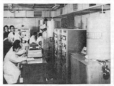
A China-made hydrogen maser for time frequency standard is important in astronomy, communication, navigation and satellite tracking as well as high precision timekeeping.
