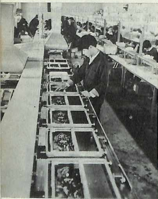
Imported automatic welding machine processes radio-cassettes in joint-venture plant. Photos by Zhu Yongqing
