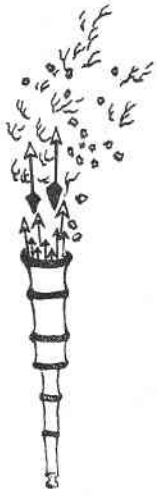
Song-dynasty "fire gun". An explosion propelled arrows and pellets, making it the predecessor of the modern gun.
