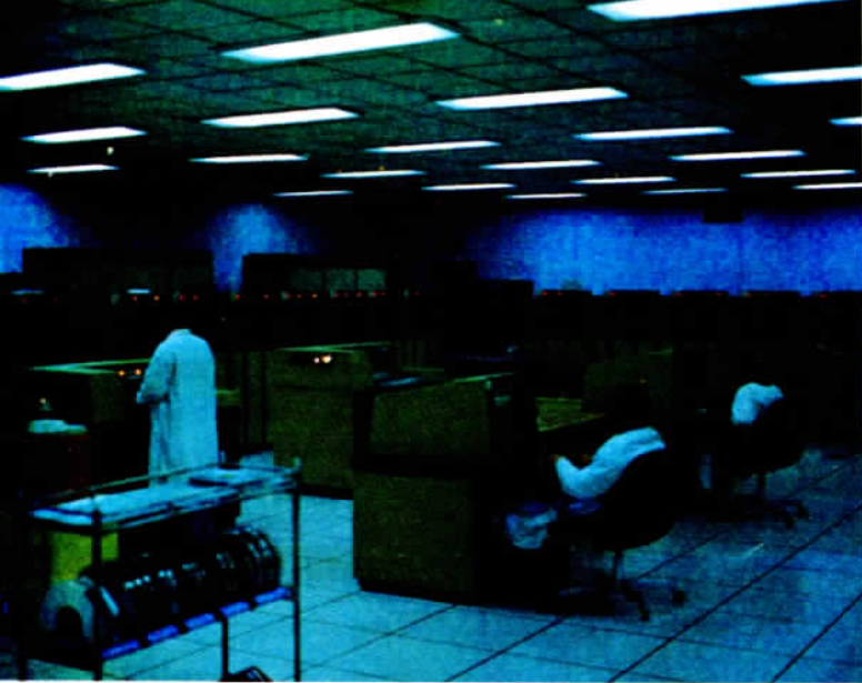
This computer centre was set up at the end of 1981 in the Zhanjiang oil base area. The large vector computer system is capable of handling one million operations a second. Photo by Xu Jun
