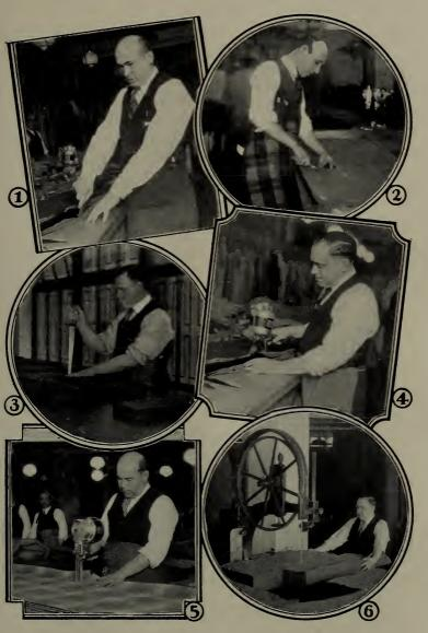
1. Jigger Knife. 2. Short Knife. 3. Long Knife. 4. Round Wheel, Machine. 5. Up and Down, Machine. 6. Bandsaw Machine.
